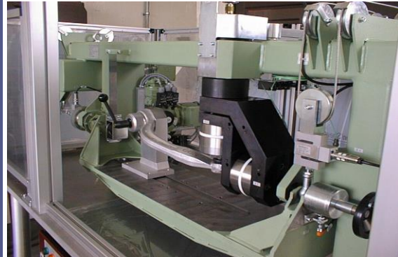
Friction Moment Measuring RMM-1422 with hydraulic clamping
