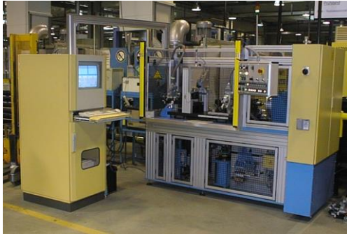
Semi-automatic elasticity measuring machines EMM-1423 for automobile suspension joints
