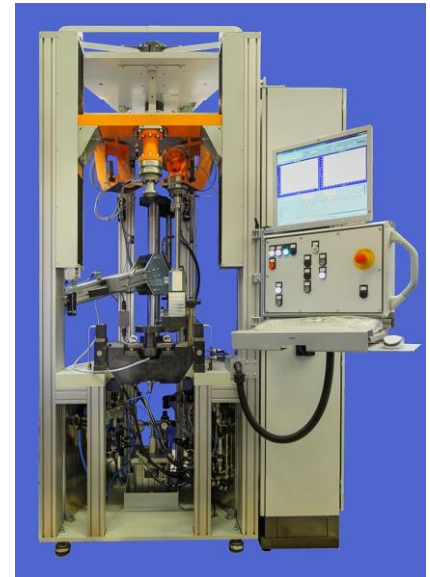
Elasticity measuring machines with hydraulic clamping and additional measuring chain for free clamping
