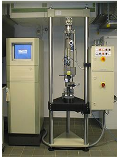
Elasticity measuring machines EMM-1291 for automobile suspension joints with hydraulic clamping
